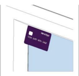
To correctly locate the brackets, take a standard sized debit or credit card and hold it in the corner of the glass.
