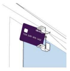
Slide the bracket into place so that it's lined up with the edge of the card. Do the same on each side, top and bottom.
