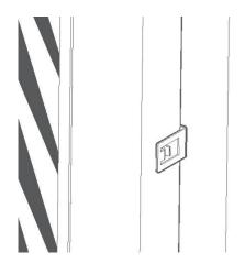
Taller shutters may be fitted with a 'midrail' to increase the shutter panel's stability.
