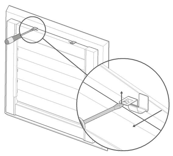
If at any point you need to remove the shutter from the window, for example to clean your windows, then it's easy; just use a flat head screwdriver or another slim, blunt object to gently pry the brackets free of where they clip into the shutter. Loosen the brackets at the top, then at the sides (if you have a taller shutter with side brackets), then tilt the top of the shutter toward you and lift away from the window.
